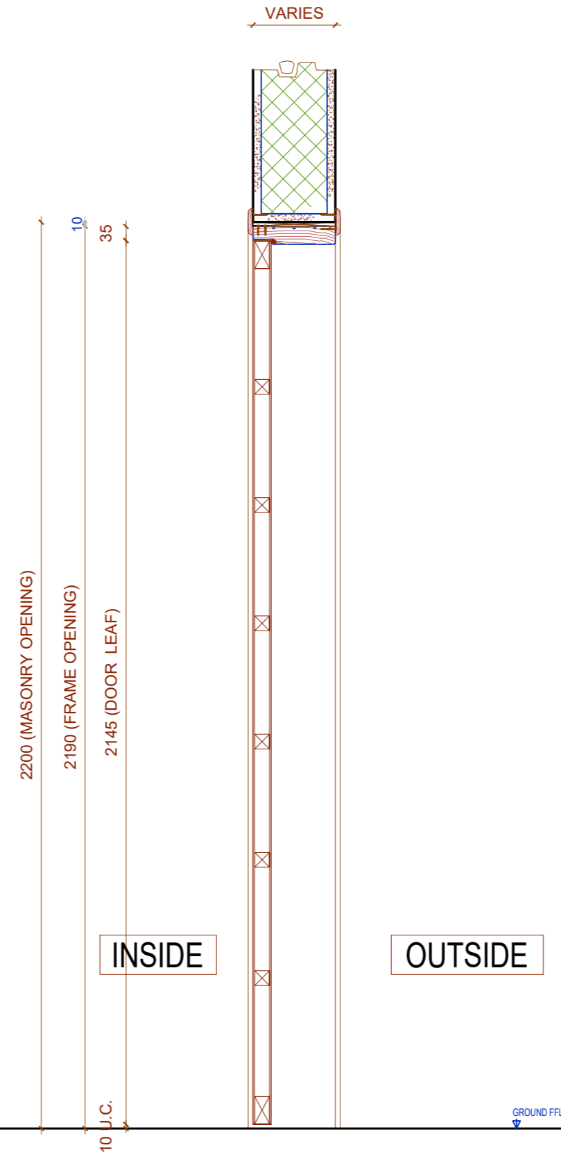
3 HOLLOW CORE WOOD TYP. SECTION SCALE 1:10
