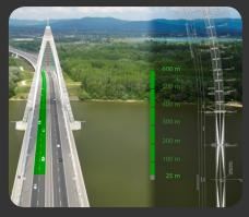
Valid speed detection at 600 m / 1970 ft, ANPR/LPR up to 150 m / 490 ft even during nighttime.
