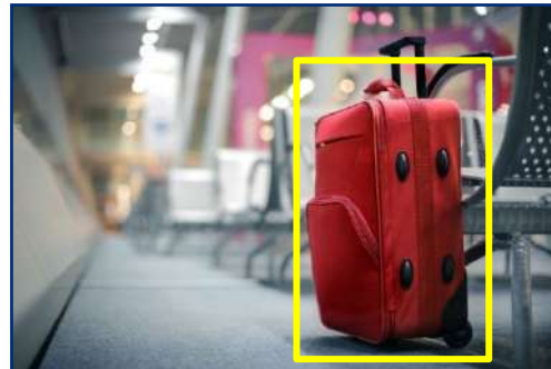
Object detection allows user to identify an object unattended for longer than a predefined time
