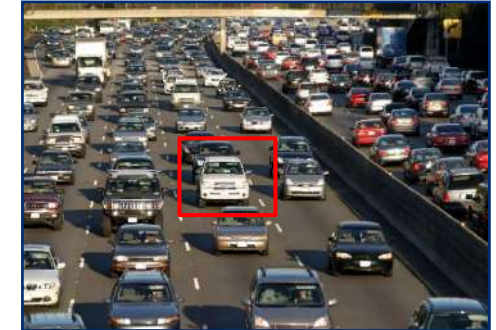
Stopped vehicle detects a vehicle stopped in a predefined area
